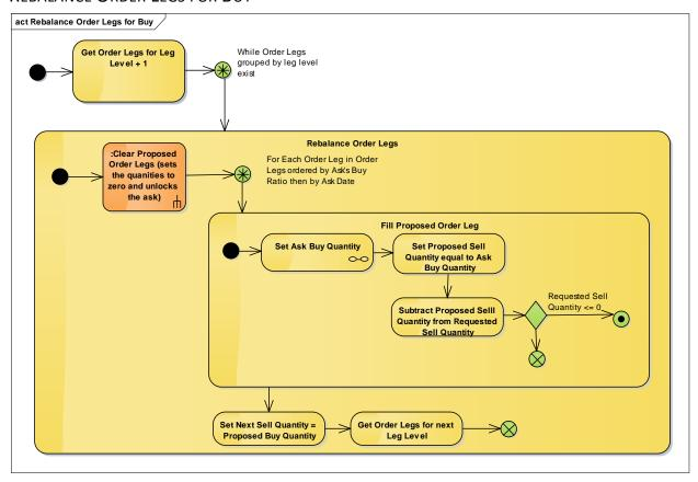
The rebalance starts by fetching the Proposed Order Legs for the previous level and then entering a loop that will iterate over all previous Proposed Order Legs grouped by leg level.
